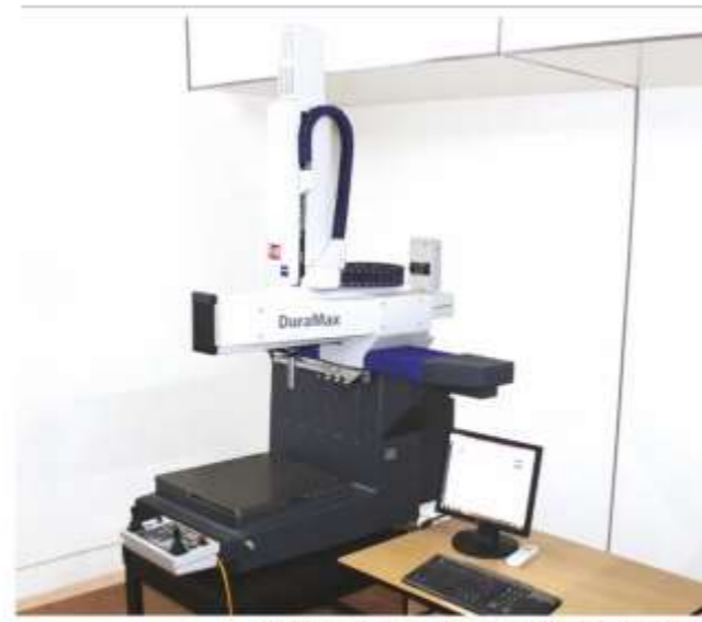
QUALITY CONTROL USING MODERN CMM
