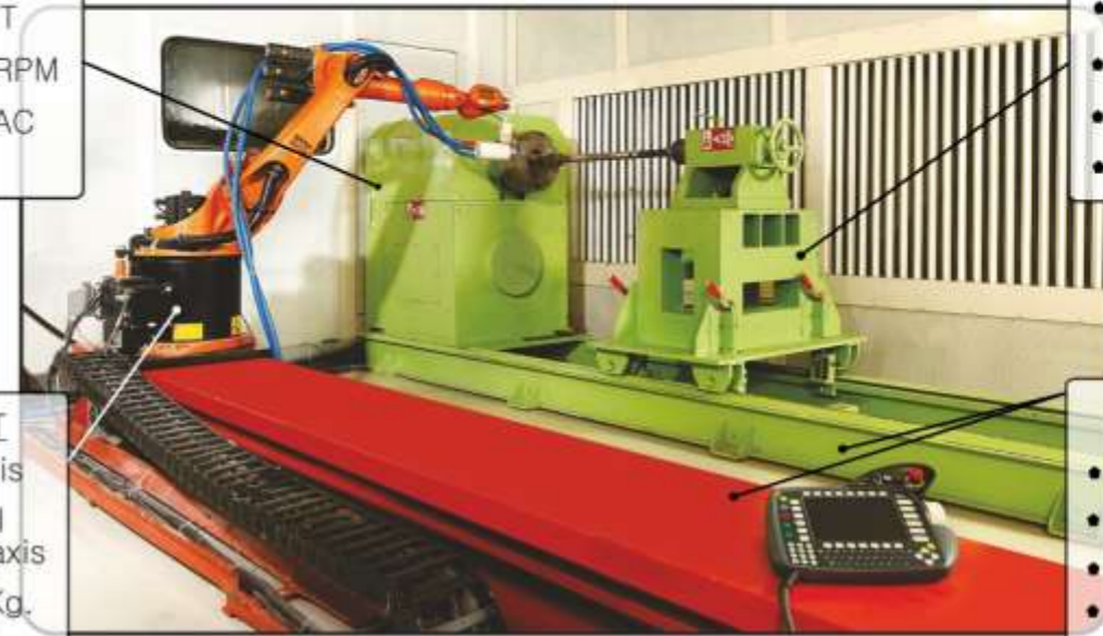
6 AXES ROBOT WITH 7 TH AXIS LINER TRACK
