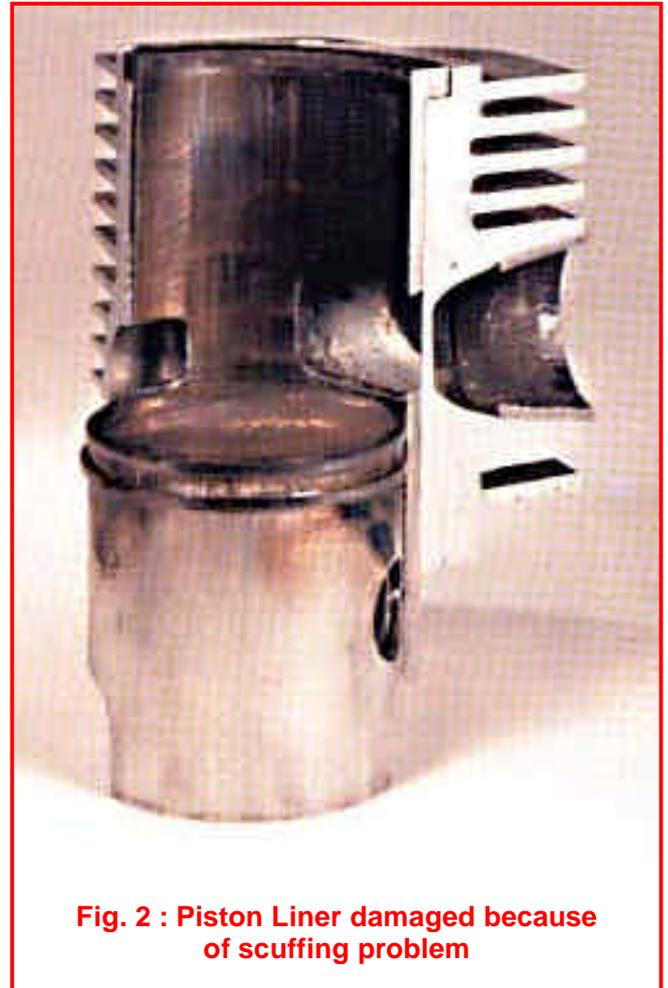
**Fig. 2 : Piston Liner damaged because of scuffing problem**
