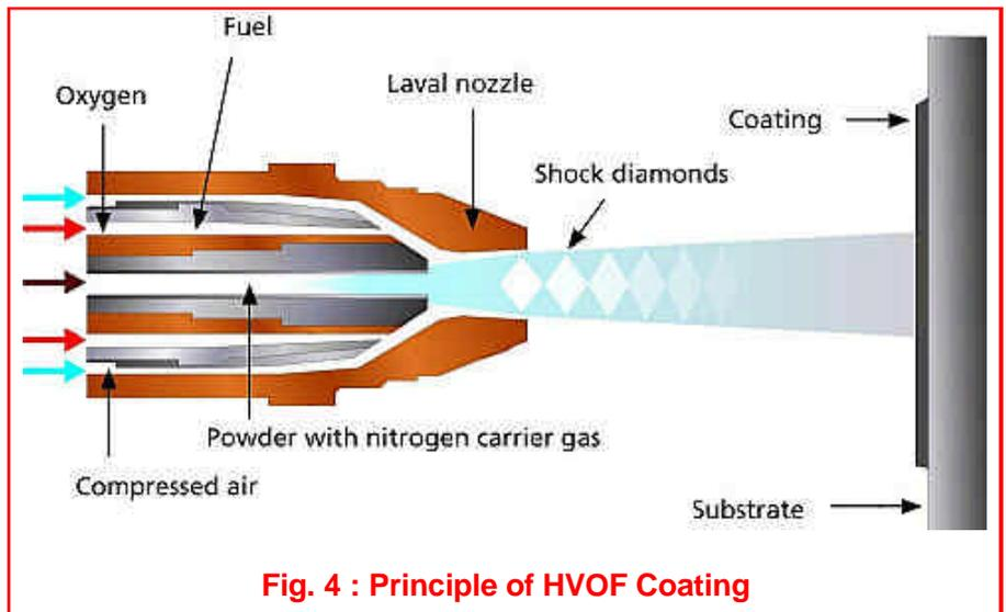
**Fig. 4 : Principle of HVOF Coating**
