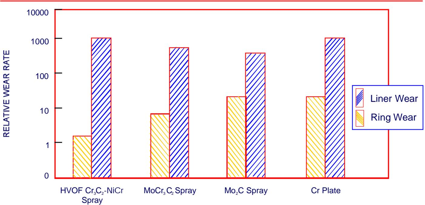
**Fig. 3 : Summary of the piston ring coating and cylinder liner wear results under steady state condition engine tests comparing thermally sprayed coatings and electroplated chromium**
