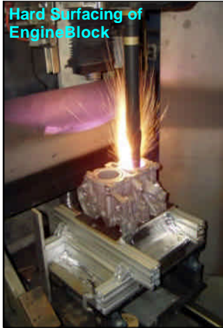
HVOF Coating for hard surface
