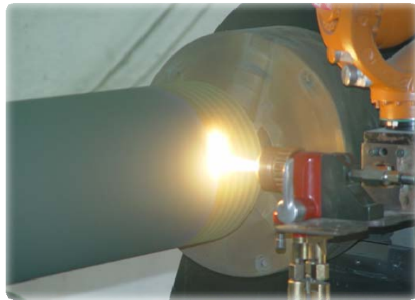
Ceramic coating on CAL roll
