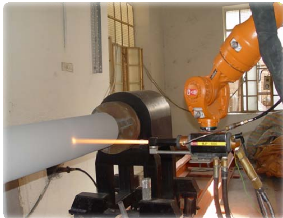
HVOF coating on Sink roll
